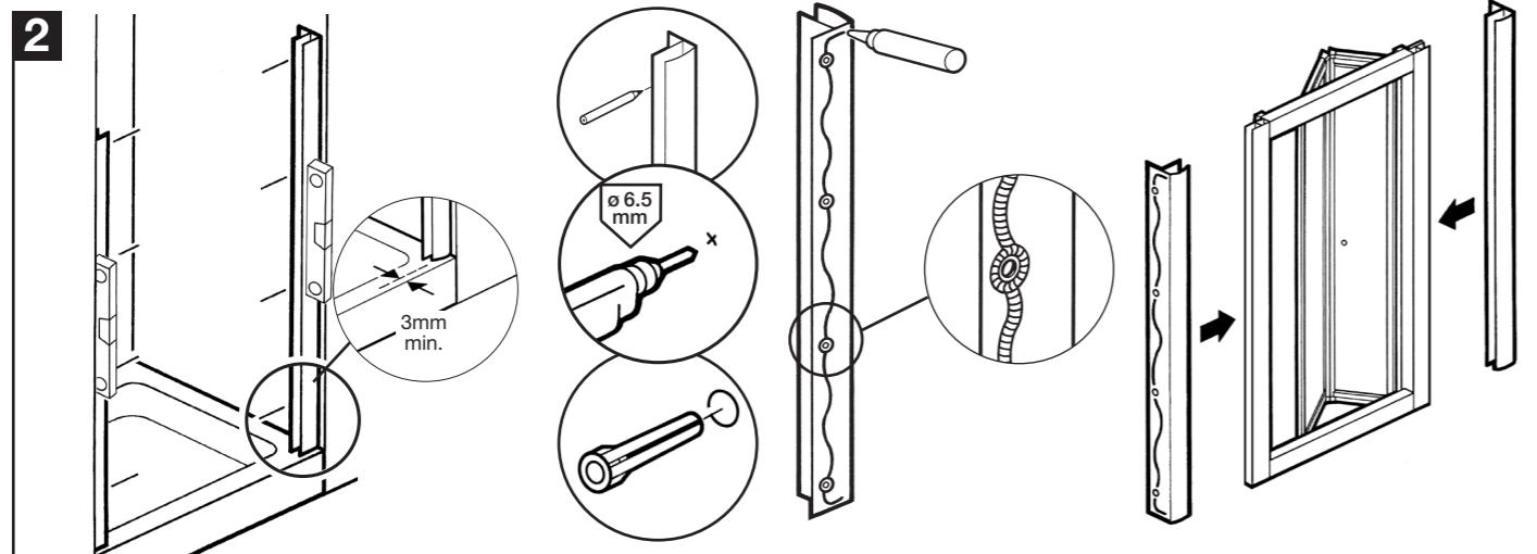
**GB** Place wall channels on tray ensuring they are vertical and a minimum of 3mm back from the front of the tray. Place masking tape against the wall before marking drill hole positions. This will help prevent the drill bit slipping. Drill 6.5mm holes, 30mm deep and insert wall plugs. Apply sealant to the back of wall channels. Place wall channels onto door.
