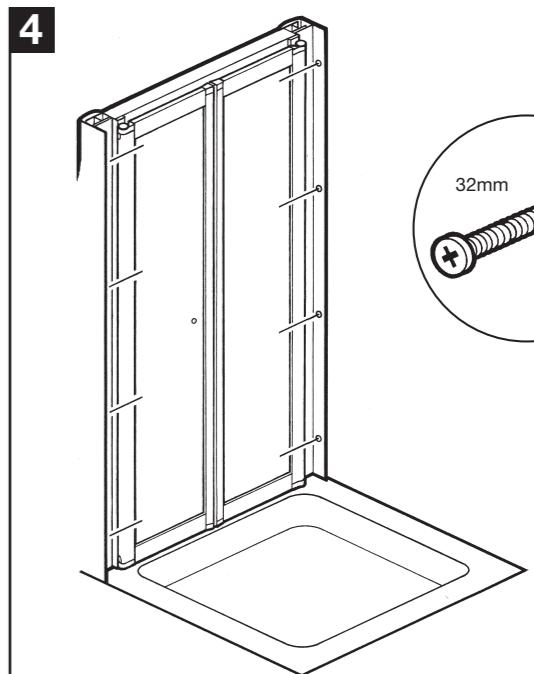
**GB** Place door in position on the tray, fix wall channels to walls using 32mm screws.
