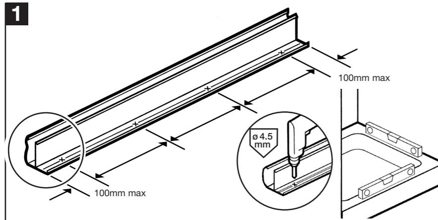
**GB** Drill holes in both wall channels at points shown using a 4.5mm drill bit, through the edge shown and between the grooves. Ensure shower tray is level in all directions.
