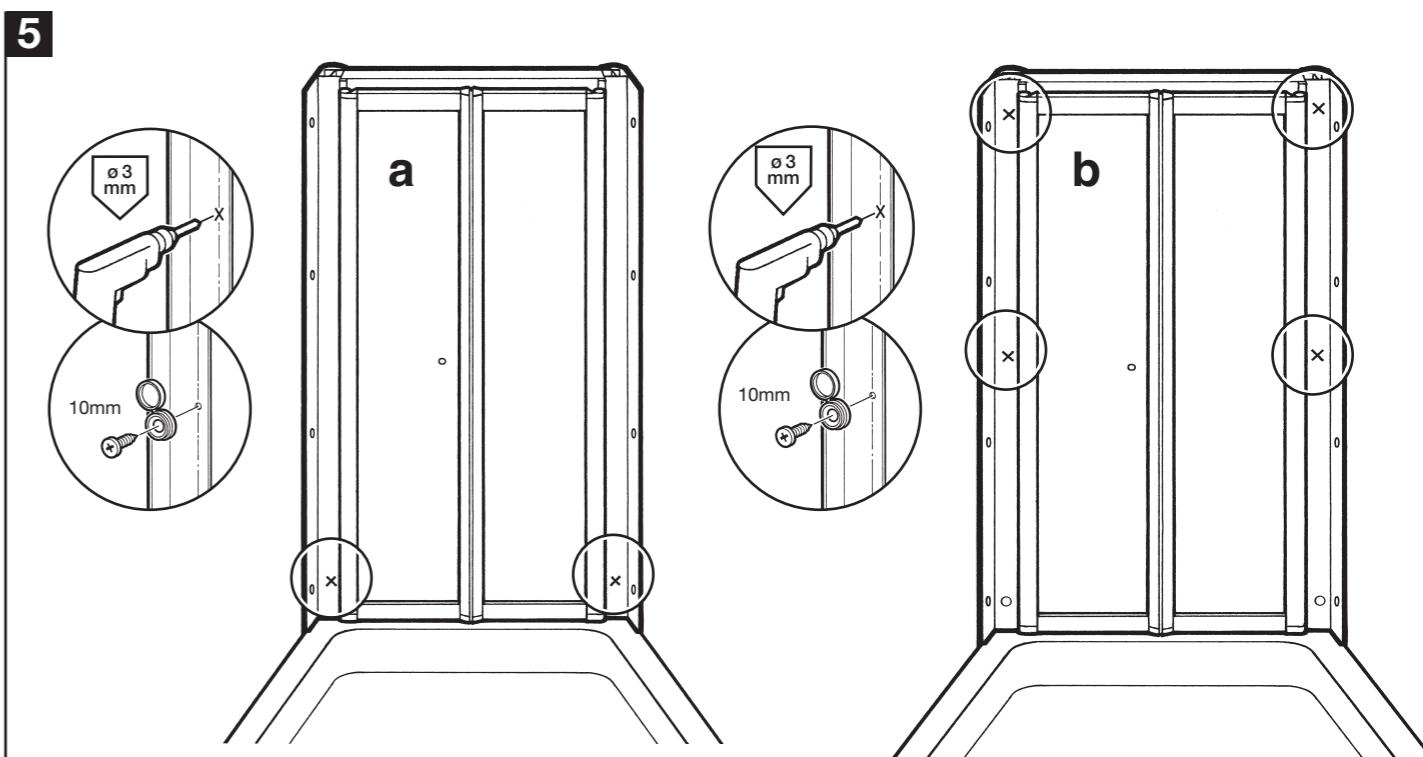
**GB** Check door is centrally positioned and perfectly vertical. Drill inside of wall channels using 3mm drill bit in the two lower positions shown. Fix using 10mm screws (a). Check door is vertical, drill next 4 holes and fix using 10mm screws (b).
