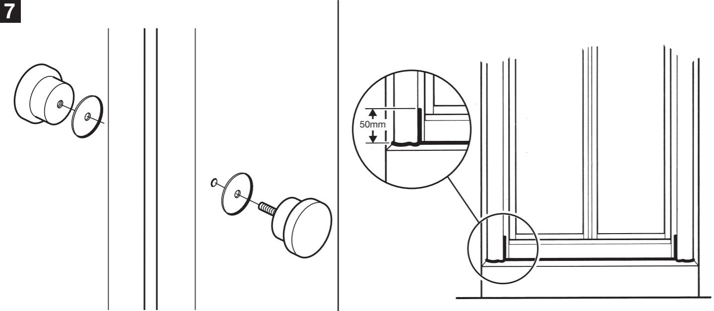
**GB** Fit door handles to the door ensuring the supplied handle washers are used on each side of the glass.
