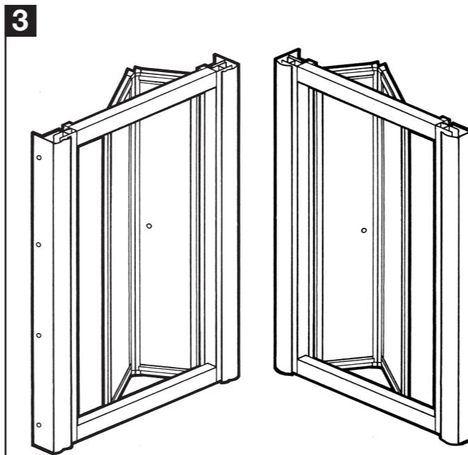
**GB** Choose which side of the door you want to fit the door handle (turn the door over if necessary).
