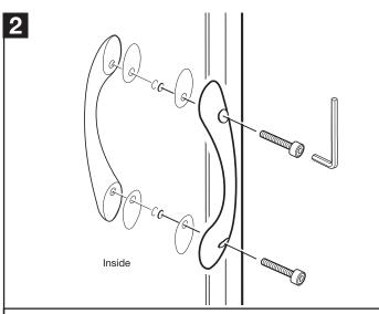
Fit the door handles to the door with the allen bolts on the inside of the door. Ensure the rubber washers are placed between the handles and the glass. **Do not over tighten.**
