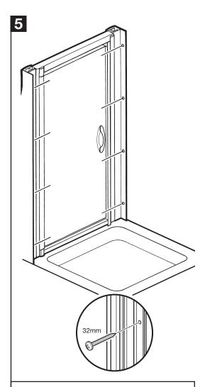
Place the door in position on the tray, fix the wall channels to the walls using 8 x 32mm screws.
